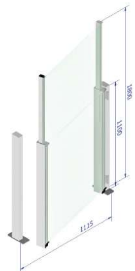
Wind Barrier wicket gate
